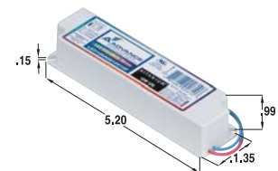
Figure C AC input: 6-inch 18AWG leads Line (black), Neutral (white) DC output: 6-inch 18AWG leads Positive (red), Negative (blue)
