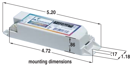
Figure A AC input: WAGO 2-pin wire trap, 18AWG solid or tinned stranded wire Line (black), Neutral (white) DC output: Use Tyco-AMP connection cable 1365323-1 (not provided)
